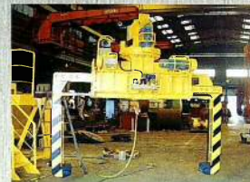
27.3t旋回CL音声ガイド付 With Audioguide System
