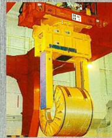
36t旋回式CL 36-ton Rotating Coil Lifter
