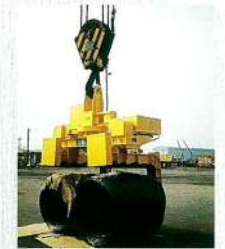
5t2個吊旋回C型フック 5-ton Rotating Twin "C" Hook
