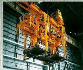
9t電動式伸縮吊ビーム (落下防止爪付) 9-ton Stretching Beam
