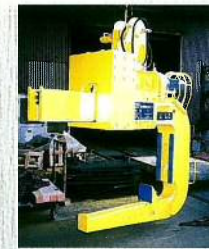
20t吊点移動式C型フック 20-ton "C" Hook With Balance Adjustment
