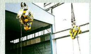
6t+6t自動玉列し吊具 Automatic Wire Disconnection Equipment
