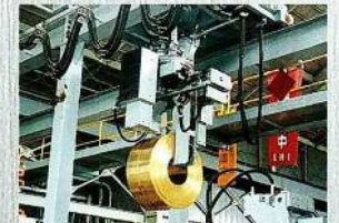
5t移動機用旋回CL For 5-ton Transfer Crane
