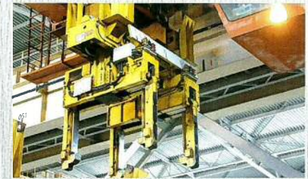
23t2ヶ吊CL自動給電装置付 23-ton Twin Coil Lifter
